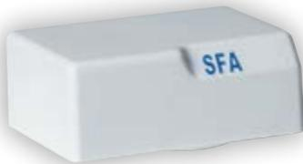
The Sanialarm has a level pressure switch that triggers an alarm fixed on the top of the unit if the volume of water exceeds the maximum allowed level. The alarm emits a continuous 80 dB warning sound until it is switched off or the problem is rectified. The Sanialarm is battery operated and can be installed on most Saniflo macerating units and drain water pumps.
